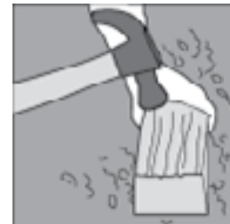
Image 2, gently tap sample can with wood block and hammer
