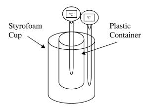
2. Fill the small container (to the top) with ice-cold water (only water, no ice!). Record the initial temperature of the water in the container.
